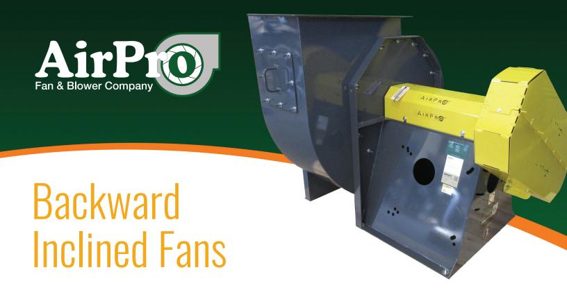
One of our most popular fan types for both induced and forced-draft applications, backward inclined fans process high volumes of air at low static pressure levels. Process air must be clean with no particulate. Designs include a non-overloading horsepower curve.
