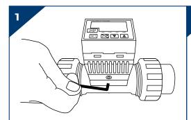
Using an allen key loosen the 2 screws located on either side of the display.
